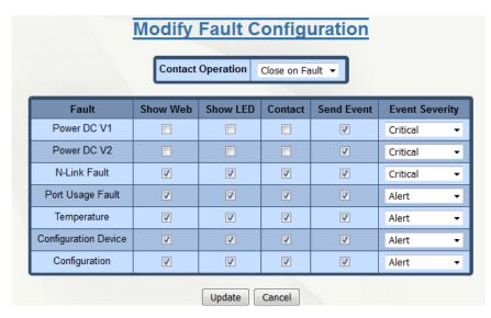
Select the desired notification settings and click on the *Update* button to save any changes. Once the save is complete, the dialog window will change to Fault Configuration.
