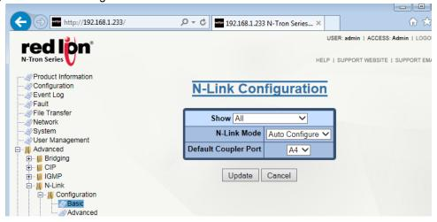
Show: View the ports that are available to install (Modules) currently installed or currently linked up.
