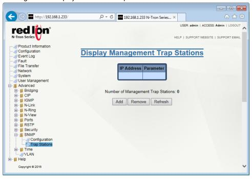
IP Address: This field represents the IP address of the Management Station to be sent SNMP Traps.
