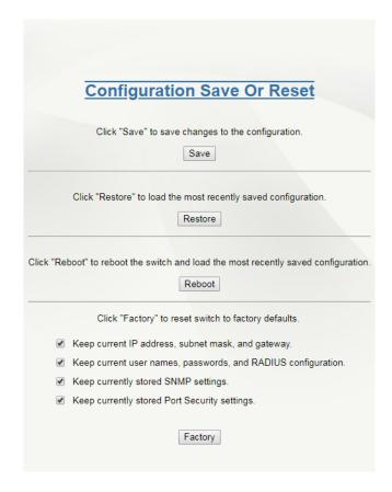
**Save:** Click on the *Save* button to save all current changes to the configuration stored in non-volatile memory for use after the next power cycle or reboot. If a configuration device is installed and enabled, the configuration will also be saved to the device. This option is only available when there is no misconfiguration.
