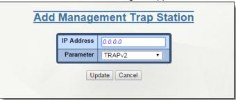
Enter the required IP address and select the parameter to be used. Click on the *Update* button and the Display Management Trap Stations screen will appear.
