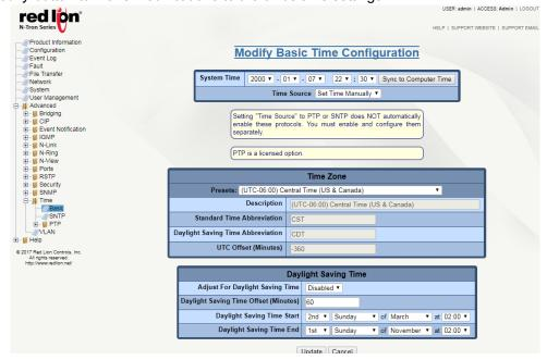
**System Time:** This field displays the date/time of the system. The system date/time defaults to 2000-01-01 00:00:00 CST (UTC-06:00) at system start. The system date/time can be set manually but in the event of a power cycle or reboot it will revert to the default value.
