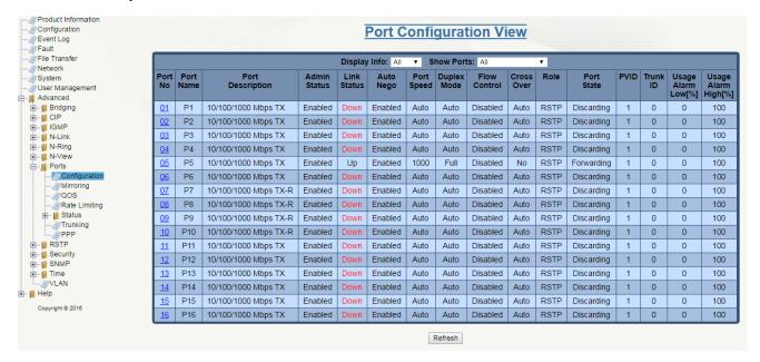
The screen above represents the Port Configuration View for a PoE model. If not using a PoE model, the page will be similar except the PoE Status column will not be present.
