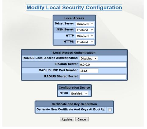
These settings address local access to the switch. For better security, keep the Telnet Server and HTTP disabled.
