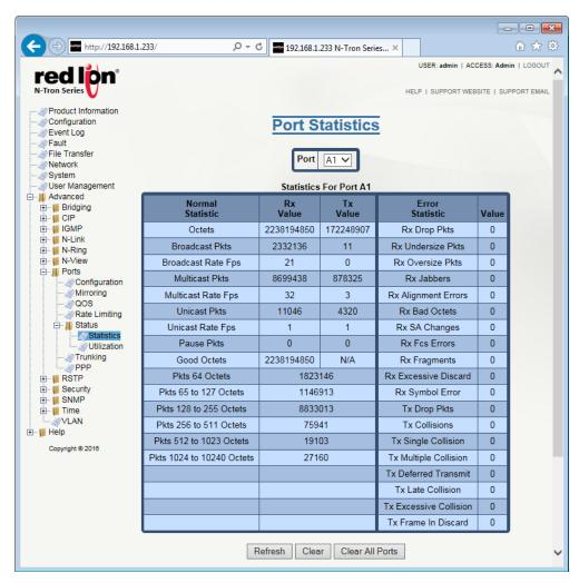
Pressing the *Clear* button resets all counters for the selected port. The *Clear All Ports* button resets all counters for all ports, including the selected port. The *Refresh* button reloads the dialog window.
