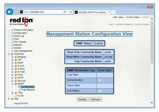
**SNMP Status:** This field indicates whether SNMP is enabled or disabled.
