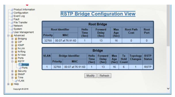
Root Bridge: This is the identity and parameters of the RSTP Root Bridge.
