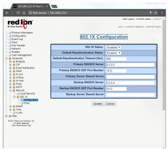
**802.1x Status:** This field indicates whether the 802.1x feature is enabled or disabled. At least one RADIUS server must be specified for 802.1x to be enabled. Ports must also be individually enabled on the ports configuration page.
