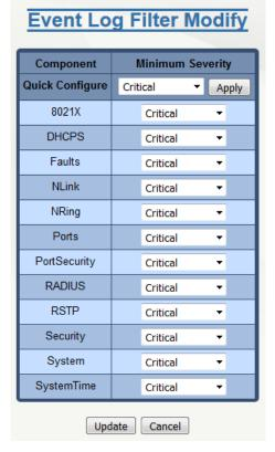
Quick Configure: Use Quick Configure to change all components to the same severity level.
