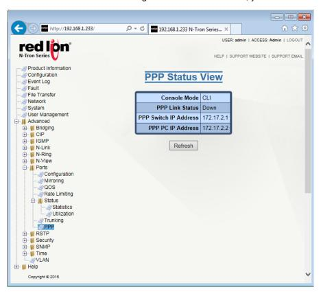
**Console Mode:** When CLI is shown, the console is in the command mode, which is the default mode. When PPP is shown, the console is in PPP mode.
