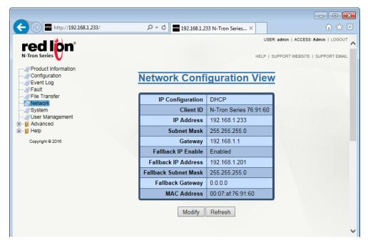
**IP Configuration:** Determines the method used to obtain an IP address, Subnet Mask, and Gateway address. When Static is selected, the statically configured values are used. When DHCP is selected, DHCP protocols are used to obtain these values.
