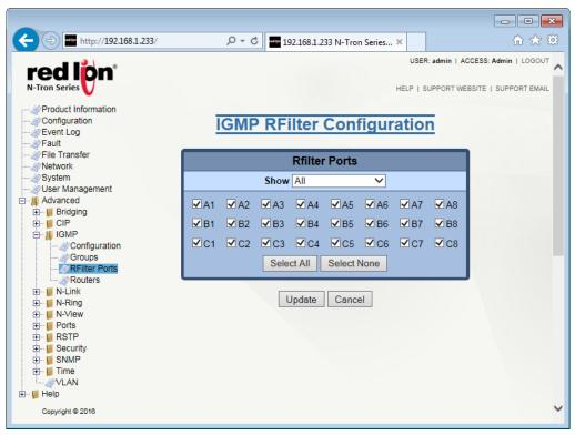
From this dialog window, the administrator selects which ports to identify as RFilter ports and can view all possible ports (Modules), currently installed ports or currently linked up ports. Click on the *Update* button when done with required changes. To save the changes made, return to the Configuration menu and click on the *Save* button.
