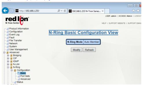
Click on the Modify button to make changes to the N-Ring Basic Configuration:
