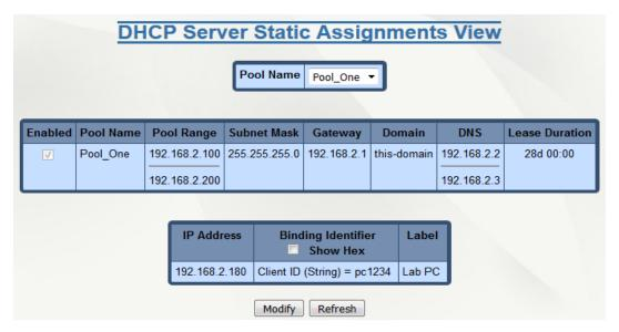
Select the Pool Name drop-down list to filter on a specified pool.
