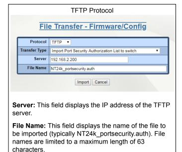
Import Port Security Authorization List to switch: Select which configuration settings to keep when the new configuration file is imported by checking on the relevant checkbox.
