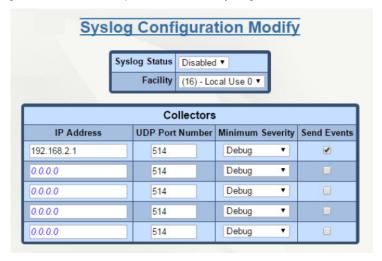
**Syslog Status:** This field indicates whether the Syslog Distributor (client) has been enabled or disabled. To enable Syslog at least one Syslog Collector (server) must be specified.
