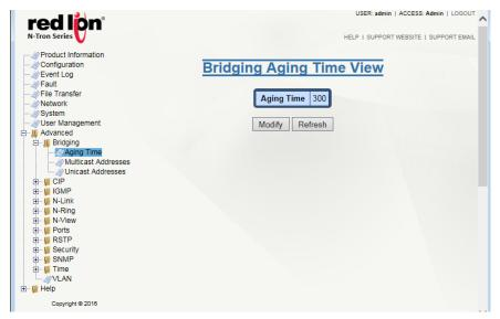
To modify the Aging Time field, click on the *Modify* button. Enter the desired Aging Time (value must be between 10 - 630 seconds) and click on the *Update* button. The default value for this field is 300 seconds. To save the changes made, return to the Configuration menu and click on the *Save* button.
