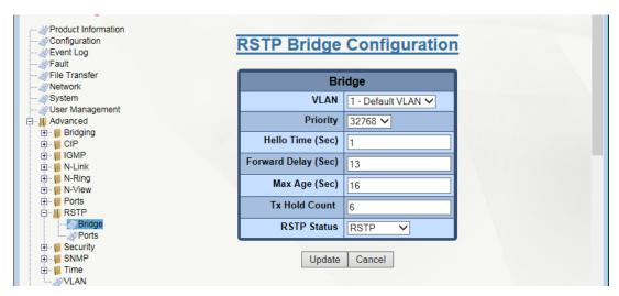
Make the required modifications, and click on the *Update* button. To save the changes made, navigate to the *Configuration* menu and click on the *Save* button.Ports
