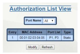
The Modify button allows the administrator to add new MAC addresses, and to modify and remove existing MAC addresses. The last row is used to add new MAC addresses and to change the ports of an existing MAC address.
