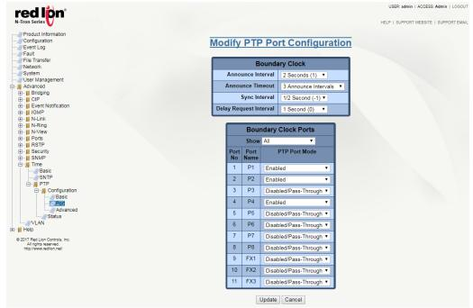
Once modifications to Announce Interval, Announce Timeout, Sync Interval, Delay Request Interval or PTP Port Mode have been made, click on the *Update* button.
