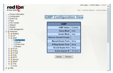
**IGMP Status:** This field indicates whether the IGMP is enabled or disabled. The default value for this field is *Enabled*.
