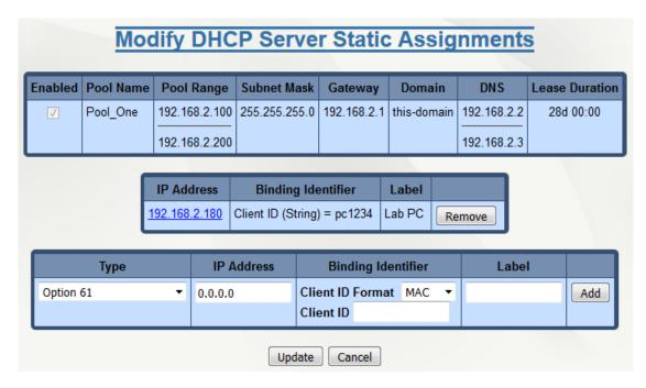
Click on the IP address hyperlink to modify the corresponding static assignment.
