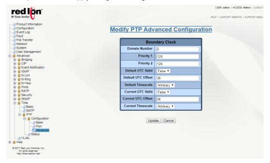
**Note:** The settings on the PTP Advanced Configuration View page are associated with the mode set on the PTP Basic Configuration View page.
