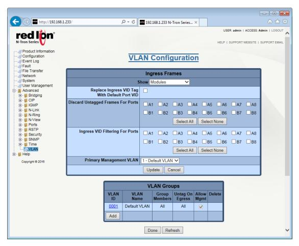
The top table is used for general VLAN changes. Once the required changes have been made, click on the *Update* button and then go to the Configuration menu and click on the *Save* button to ensure all changes are saved.
