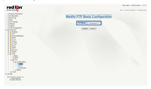
**Note:** When switching between PTP modes, it will be necessary to save the configuration and reboot the switch for changes to apply.
