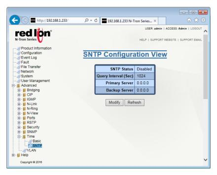
**SNTP Status:** Indicates whether the SNTP client has been enabled. In order to enable SNTP, at least one SNTP or NTP server must be specified.
