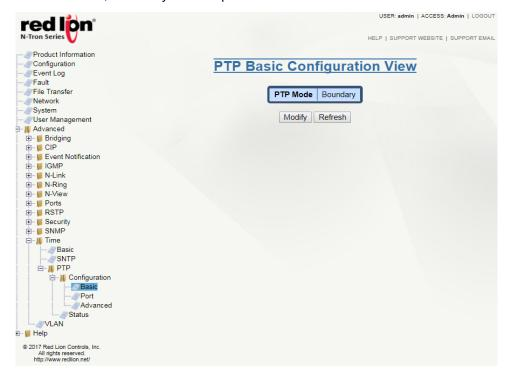
**PTP Mode:** This field indicates whether PTP is disabled, operating as a Boundary clock, or operating as a Transparent clock.
