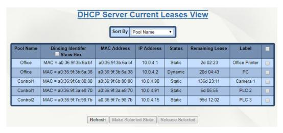
**Sort By:** Sort the current leases by Pool Name, Binding Identifier, MAC Address, IP Address, Status, Remaining Lease, or Label.
