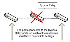
**Note:** It is still possible to customize port settings in any configuration desired, based on network requirements. Network testing must be performed to ensure correct network operation whether the switch is powered on or powered off.
