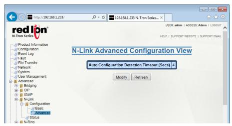
Click on the *Modify* button to change the detection timeout. Click on the *Update* button once the field has been updated with the required information. To save the changes made, return to the *Configuration* menu and click on the *Save* button.
