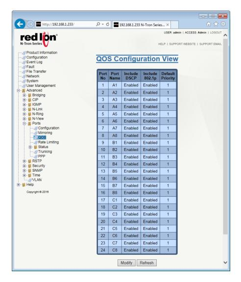
**Include DSCP:** This configurable field displays the status of whether or not to include the ingress frame's RFC 2474 DSCP value in determining the transmit priority and egress frame's IEEE 802.1p User Priority value. If the ingress frame type is IP (IPv4 or IPv6) and Include DSCP is enabled, DSCP processing will override all other settings. (see QOS SELECTION CHART below). The default value is enabled.
