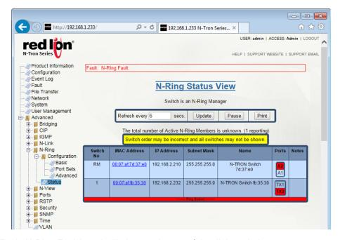
A fault warning Fault: N-Ring Fault in red will show at the top of the dialog window.
