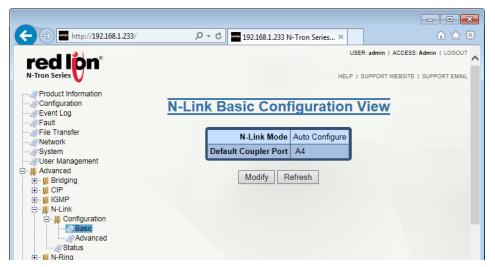
Click on the *Modify* button to make changes. Click on the *Update* button to retain the changes. To save the changes made, return to the Configuration menu and click on the *Save* button.
