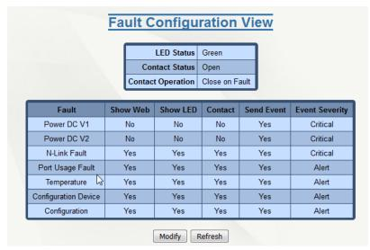
**LED Status:** This field shows the current color of the Power/Fault LED. Green indicates there is no fault and Red indicates a fault condition exists.
