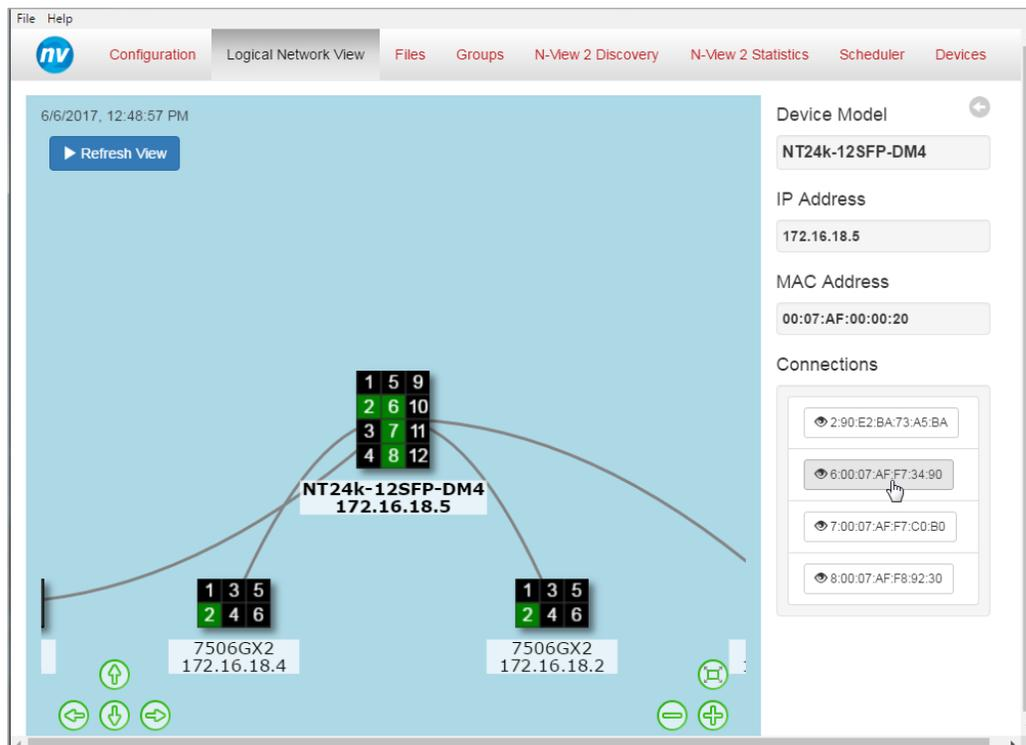
By clicking on the MAC addresses listed in the connections section of the device information panel the corresponding device is selected in the logical network view and the device information is updated.
