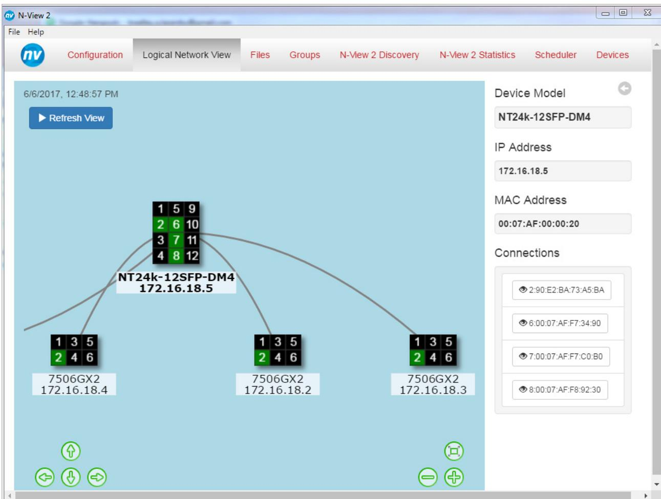
The network view displayed corresponds to the last time a network discovery was performed. The time of the last Network Discovery is displayed in the top left corner.
