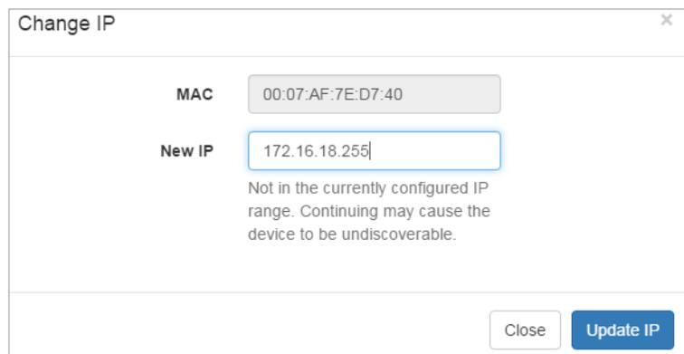
The dialog box titled "Change IP" contains a "MAC" field with the value "00:07:AF:7E:D7:40" and a "New IP" field with the value "172.16.18.255". Below the "New IP" field, the error message "Not in the currently configured IP range. Continuing may cause the device to be undiscoverable." is displayed. At the bottom right, there are "Close" and "Update IP" buttons.
