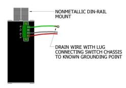
If the use of shielded cables is required, it is generally recommended to only connect the shield at one end to prevent ground loops and interfere with low level signals (i.e. thermocouples, RTD, etc.). Cat5e cables manufactured to EIA-568A or 568B specifications are required for use with N-Tron Switches.
