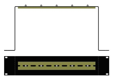
Most N-Tron<sup>TM</sup> products are designed to be mounted on industry standard 35mm DIN rail. However, DIN rail mounting may not be suitable for all applications. Our Universal Rack Mount Kit (P/N: URMK) may be used to mount the 100-POE4 enclosures to standard 19" racks as an option.
