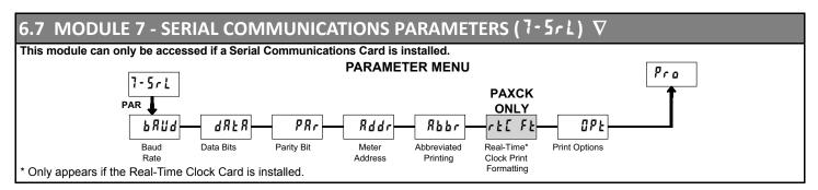
Module 7 is the programming module for the Serial Communications Parameters. These parameters are used to match the serial settings of the PAX with those of the host computer or other serial device, such as a terminal or printer. This programming module can only be accessed if an RS232 or RS485 Serial Communications card is installed.
