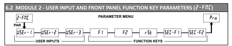
Module 2 is the programming module for the rear terminal User Inputs and front panel Function Keys.
