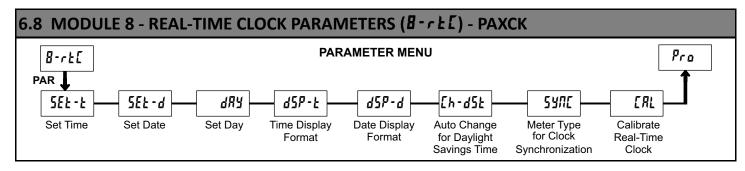
Module 8 is the programming module for the Real-Time Clock (RTC) Date and Time Parameters. In the Display Mode, the DAT annunciator indicates the RTC Date is currently being shown. The RTC Time display is shown with no annunciator. This programming module can only be accessed if a Real-Time Clock card is installed.
