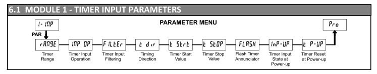
Module 1 is the programming module for the Timer Input Parameters. In the Display Mode, the **TMR** annunciator indicates the Timer display is currently being shown. An **EXCHANGE PARAMETER LISTS** feature, which includes the Timer Start and Timer Stop Values, is explained in Module 2.
