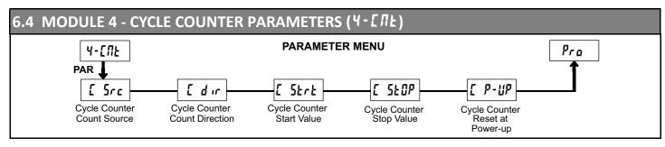
Module 4 is the programming module for the Cycle Counter Parameters. In the Display Mode, the CNT annunciator indicates the Cycle Counter display is currently being shown. An **EXCHANGE PARAMETER LISTS** feature, which includes the Cycle Counter Start and Stop Values, is explained in Module 2.
