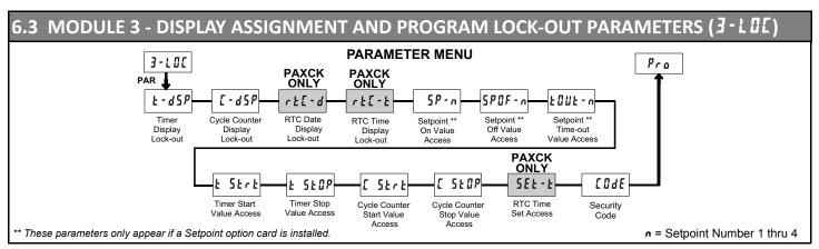
Module 3 is the programming module for setting the Display Lock-out Parameters and the "Quick Programming Mode" Value Access Parameters. In the Quick Programming mode, after the PROGRAM LOCKOUT PARAMETERS and before the Security Code (fild), a Display Intensity Level (d-lf) parameter is available when the security code is non-zero. It allows the display intensity to be set to 1 of 16 levels (0-15).
