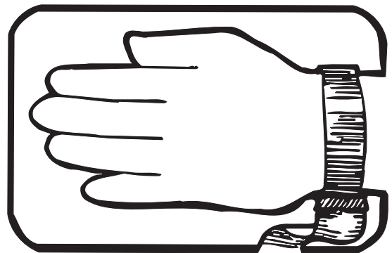
3. DISCHARGE PERSONAL STATIC BEFORE HANDLING DEVICES. USE A HIGH RESISTANCE GROUNDING WRIST STRAP.
